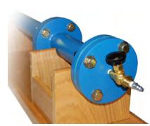
K9901C Instrumented Shock Tube for Pressure Sensors A number of national metrology institutes including NIST, LNE and NPL have added the capability to conduct research on dynamic pressure characterization via the well-known shock tube apparatus. For decades, PCB Piezotronics has operated this type of pressure actuator inhouse for quick rise time, high-speed
