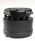
Primary accelerometer calibration is at the root of traceability for virtually every accelerometer calibration chain in the world: commercial, government, military, academic or vendor. Acceleration calibration via laser interferometry is a primary method because it is an absolute method comparing the measured vibration from a sensor under test to a constant of nature - the wavelength of laser light...
