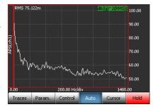
the velocity scale is too high to be "real." Ski slope is not good data and should be discarded. Many analysts make the mistake of trying to analyze this data...
