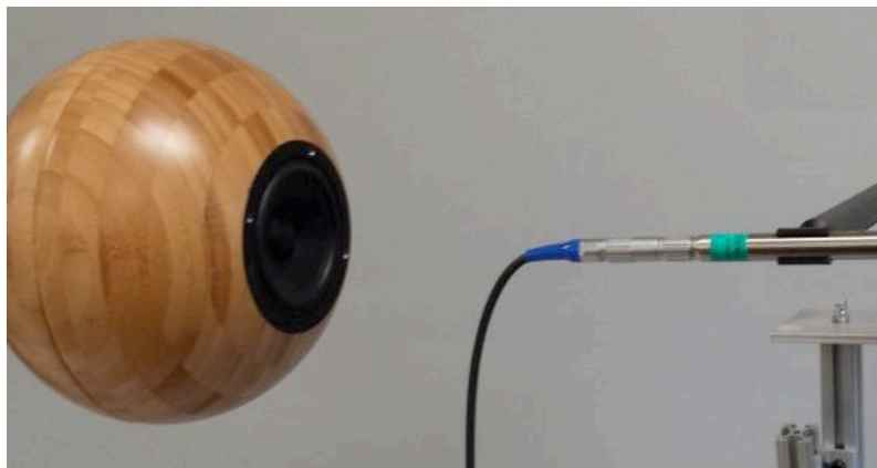
Figure 6: Speaker arranged on axis of the microphones during pressure calibration.
