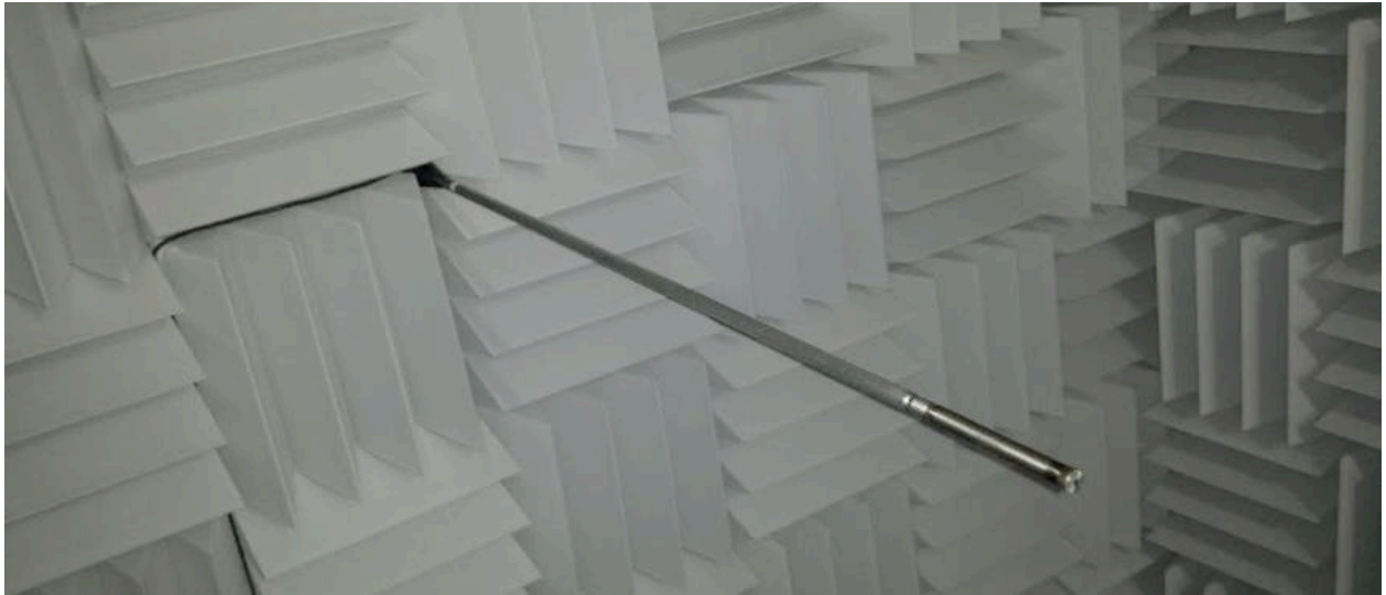
Figure 4: Wall mounted rod fixture for free field calibration.
